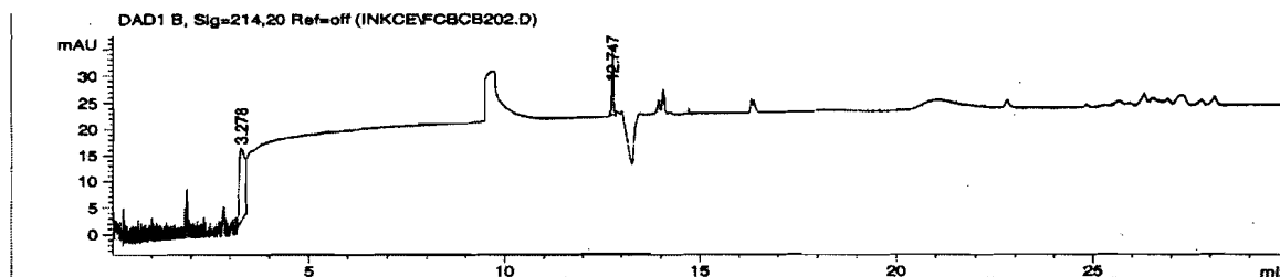
Figure 22. CE electropherogram of ink #6 extracted from 400 plugs in 200 \mu L ethanol and 200 \mu L water and run in 50mM borate buffer, pH 9.3, with 20% methanol.
