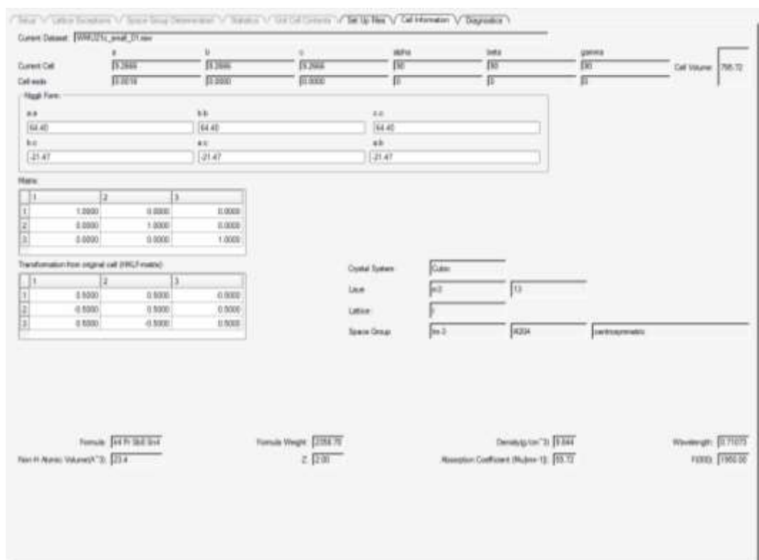
Figure 7: Displays the cell information obtained from the single crystal as found by the x – ray diffractometer.
